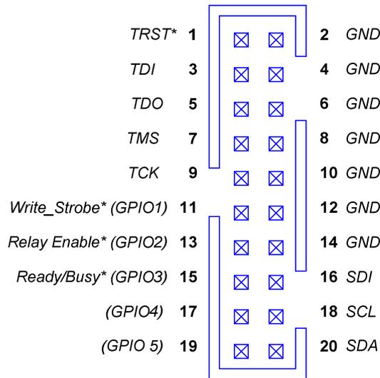
**Figure 2-2.** ScanTAP IsoPod 20-pin Controller Connector (top view)
