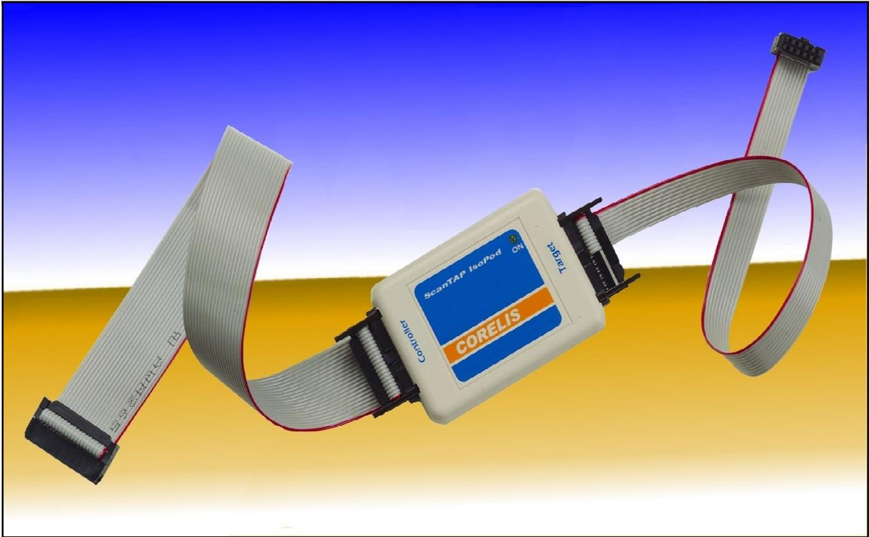
**Figure 1-1.** ScanTAP IsoPod Hardware
