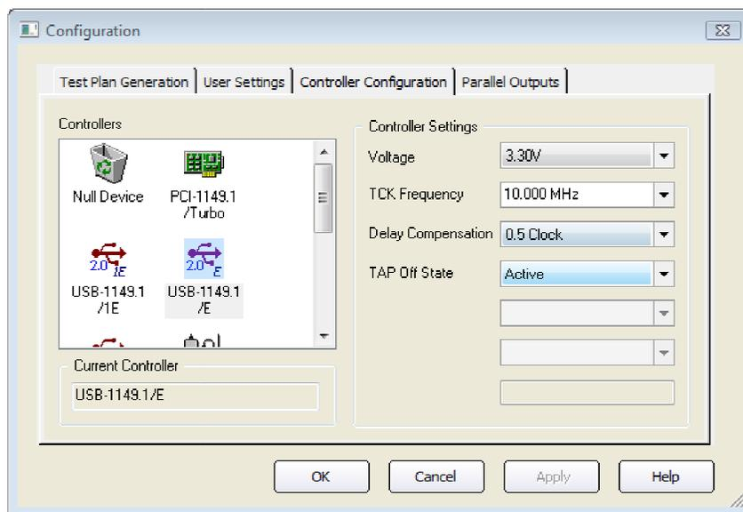
**Figure 2-4.** USB-1149.1/E Controller Configuration Screen in ScanExpress Runner
