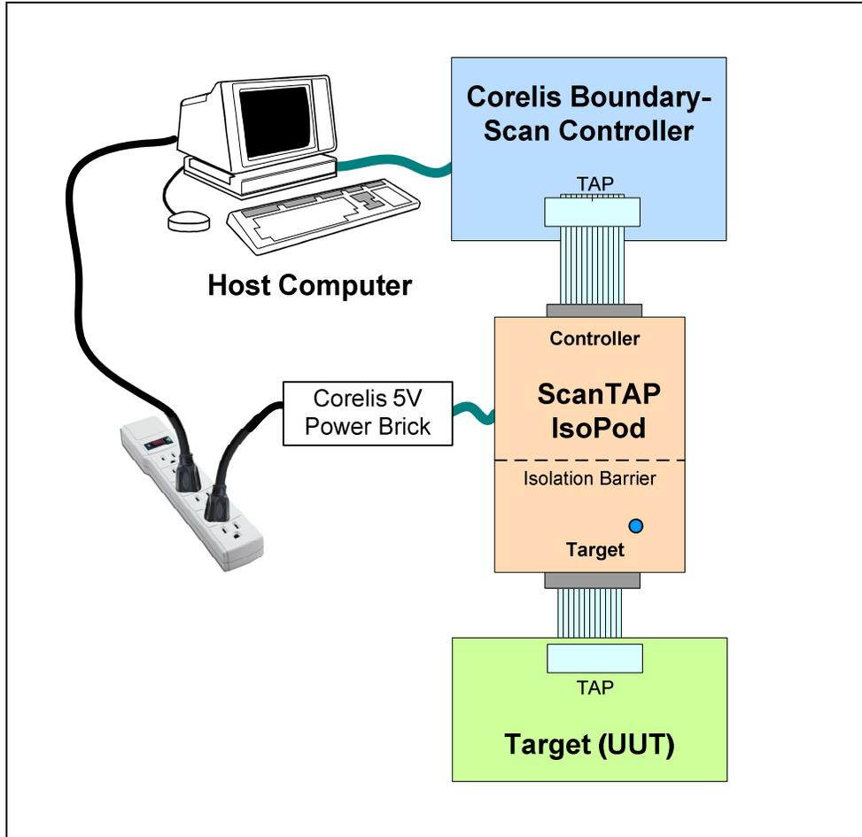
**Figure 2-1.** ScanTAP IsoPod System Connection Diagram
